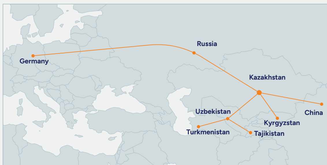
Figure 3 — Existing international fiber optic cable routes carry internet traffic from Central Asia through Russia to the rest of the global internet. This leaves Central Asia dependent on fiber optic infrastructure in Russian territory.
